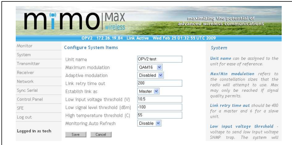
Radio Unit CCMS 'Configure System Items' page showing selection as a Master. Access is through the 'System / Configuration' tab.
